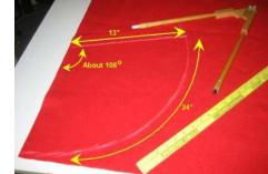
easier just to run a tape measure along the arc to measure its length.
